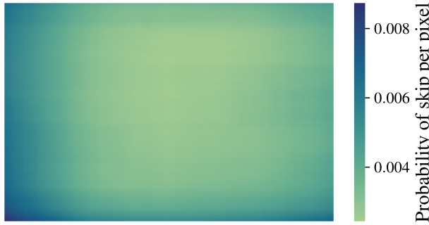
Figure 15: Dragonfly rarely experiences skipping; Skips mainly occur on the viewport edge where the impact is low.
